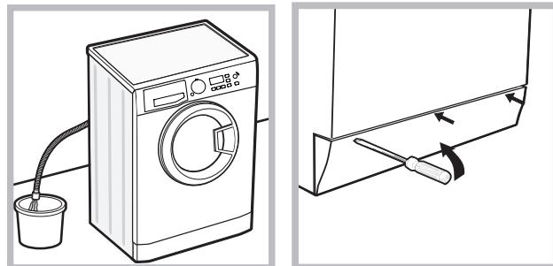
3. using a screwdriver, remove the cover panel on the lower front part of the washer-dryer (see figure).
