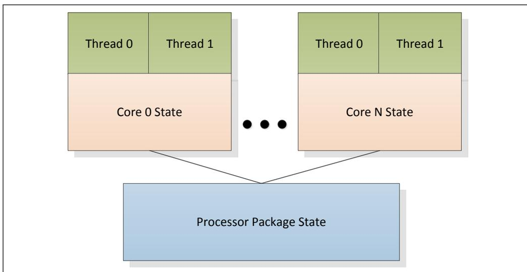
Entry and exit of the C-states at the thread and core level are shown in the following figure.
