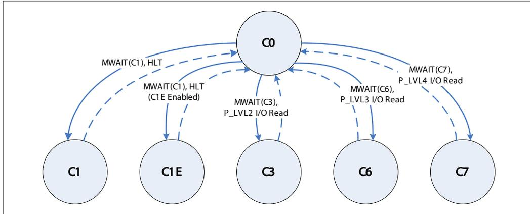
While individual threads can request low-power C-states, power saving actions only take place once the core C-state is resolved. Core C-states are automatically resolved by the processor. For thread and core C-states, a transition to and from C0 is required before entering any other C-state.
