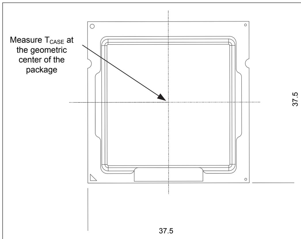
*Note:* THERM-X OF CALIFORNIA can machine the groove and attach a thermocouple to the IHS. The supplier is subject to change without notice. THERM-X OF CALIFORNIA, 1837 Whipple Road, Hayward, Ca 94544. Ernesto B Valencia +1-510-441-7566 Ext. 242 ernestov@therm-x.com. The vendor part number is XTMS1565.
