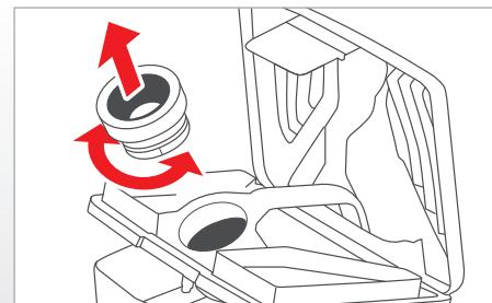
If the suction filter was removed, place it back in the waste water tank.
